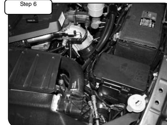
Install new tube and position into coupler on manifold. Tighten and torque all four clamps to 75 in-lbs. Check and tighten after 50 miles! Your Intercooler tube installation is now complete. Thank you for choosing aFe power!
