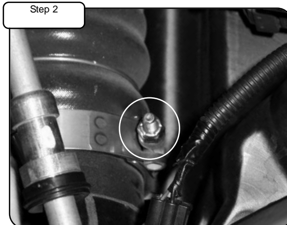
With 7/16" deep socket, loosen clamp on intercooler.
