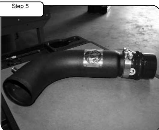
Install 3" hump coupler with clamps provided to new tube.
