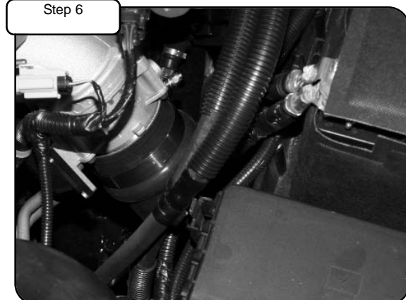
Install 3-1/2" hump coupler to manifold with clamps provided.
