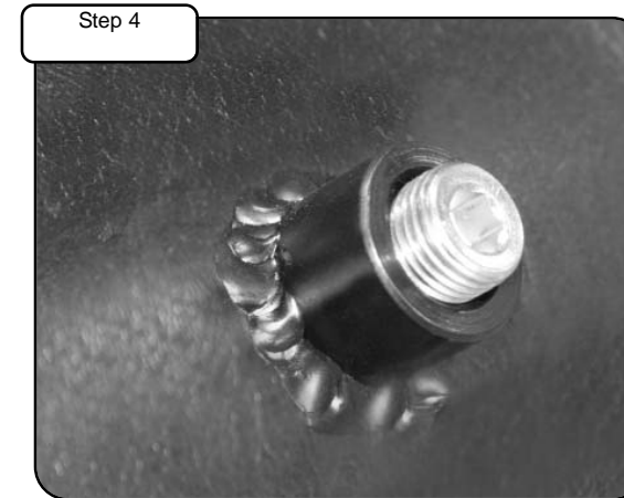
Install plugs in to 1/8" NPT ports with 3/16" hex key.
