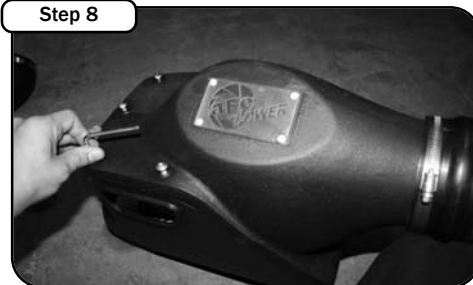
Step 8 Attach cover to bottom half of new air box and secure using the six 5/16" button head screws provided.
