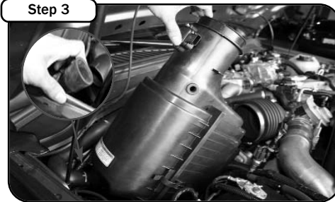
Step 3 Take auxiliary air line out of air box. Lift and pull firmly then remove OE air box out of vehicle.
