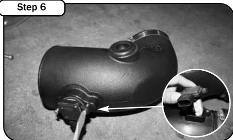
Step 6 Remove MAF sensor from stock air box using t-20 torx bit provided. Install into new tube using gasket and M4 screws and tighten using flat head screwdriver. Install grommet to hole on tube.
