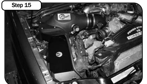
Step 15 Your installation is now complete. Make sure all hoses and clamps are tight. Check and retighten connections and filter after a few hours of operation. Thank You for choosing aFe. NOTE: Place enclosed CARB EO sticker on a clean/smooth surface near the intake system. EO identification label is required to pass the smog test inspection.
