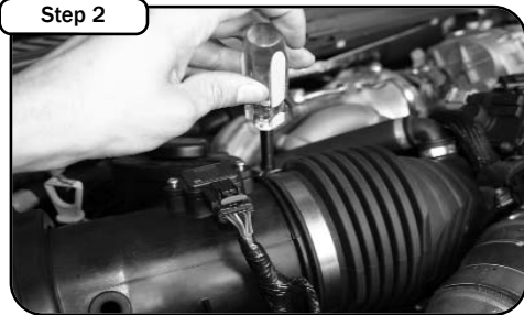
Step 2 Remove filter minder out of air box. Loosen factory clamp with 5/16" nut driver. Disconnect MAF sensor harness.
