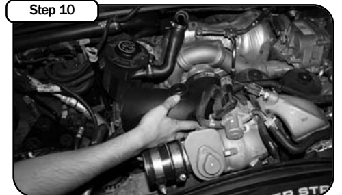
Step 10 Install new tube into vehicle and position coupler inside of tube on turbo. Note: make sure bead on coupler sits on turbo. The clamp on tube will secure the coupler inside of tube. Do not tighten.
