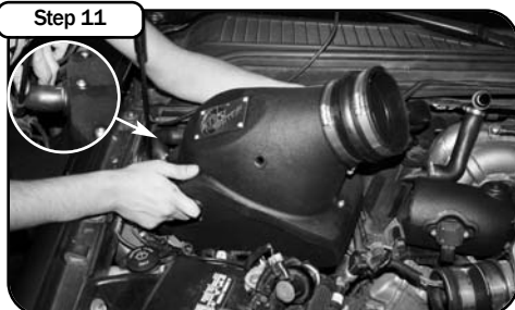
Step 11 Install intake box into vehicle and position to factory. Make sure intake box sits securely in grommets.
