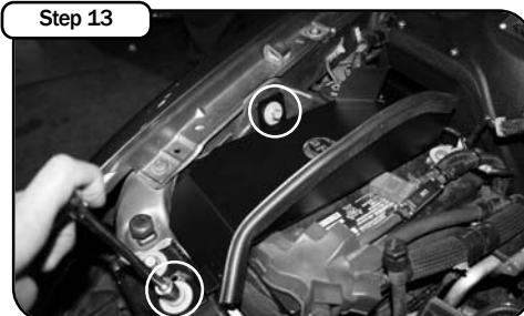
Step 13 Loosen the 2 bolts near passenger side battery for scoop install using 13mm socket or wrench. Attach trim seal to scoop and align to cut-out on housing. Re-install bolts and tighten. Note: Make sure the positive battery terminal is covered with factory cap.
