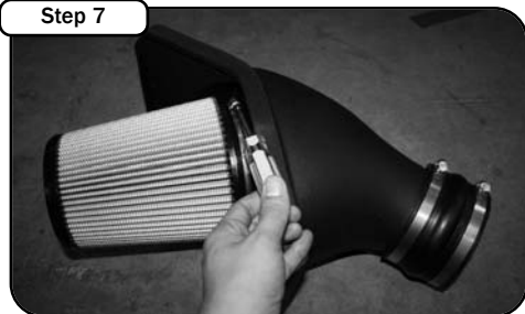
Step 7 Attach air filter to cover using 5/16" nut driver. Attach hump coupler to end of tube with clamps provided. Do not tighten.
