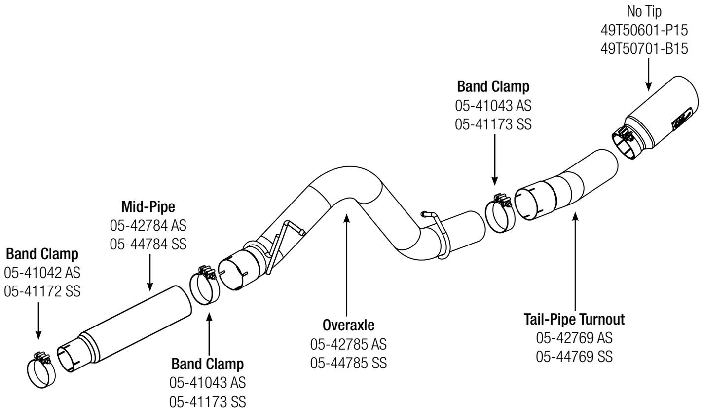
**Step 1: (Read Instructions prior to installation)** Loosen mounting flange at rear of particulate filter before muffler. Remove the stock exhaust from the rear of the truck working your way forward. Take caution not to damage the factory isolation mounts and gasket as they will be reused. **It is recommended to not fully tighten the clamps until the entire system has been installed.**
