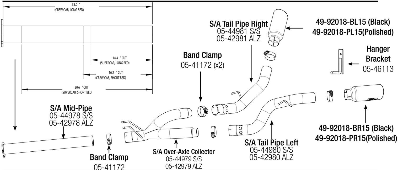
**Step 1: (Read Instructions prior to installation)** Loosen mounting flange at rear of particulate filter before muffler. Remove the stock exhaust from the rear of the truck working your way forward. Take caution not to damage the factory isolation mounts and gasket as they will be reused. It is recommended to not fully tighten the clamps until the entire system has been installed.
