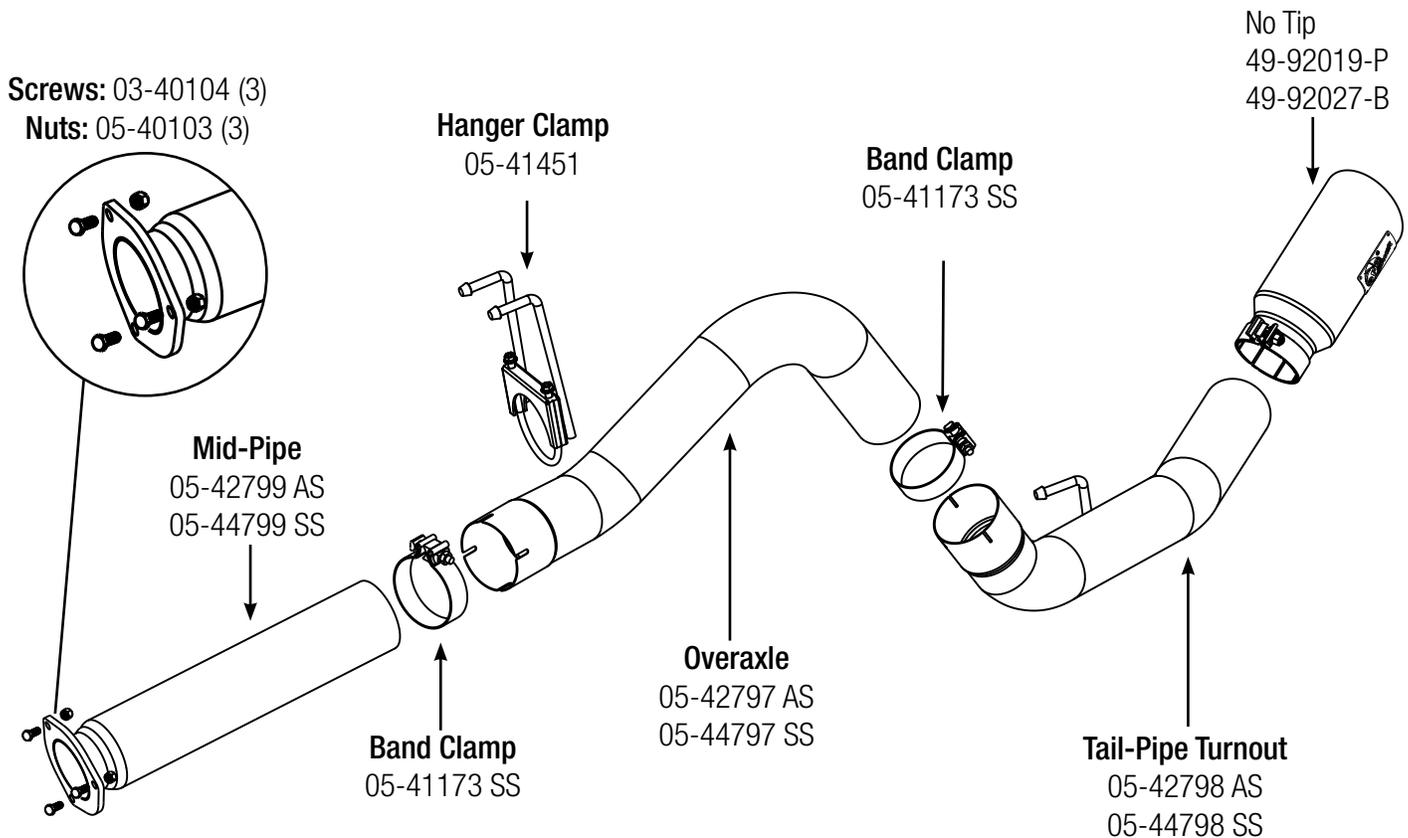
**Step 1: (Read Instructions prior to installation)** Loosen mounting flange at rear of particulate filter before muffler. Remove the stock exhaust from the rear of the truck working your way forward. Take caution not to damage the factory isolation mounts and gasket as they will be reused. **It is recommended to not fully tighten the clamps until the entire system has been installed.**
