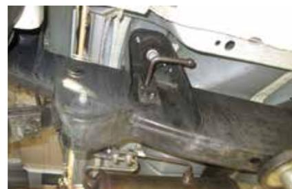
NOTES: aFe recommends that the tailpipe be at least 1/2"-1" away from any body panels to avoid heat related body damage. Tighten and secure.
