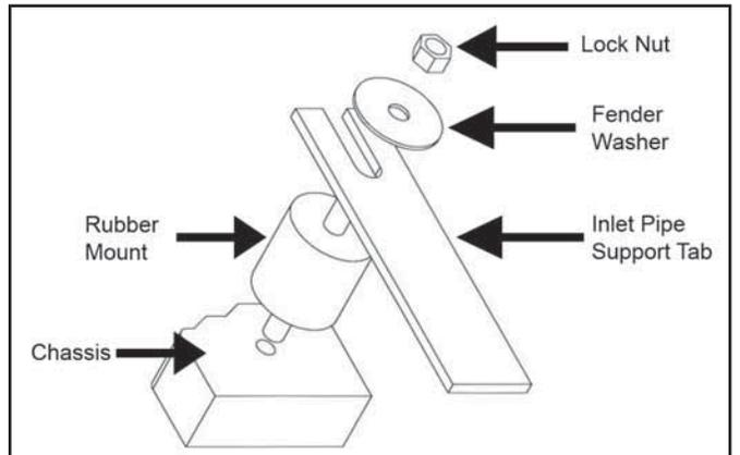
i. Diagram for proper rubber mount installation.
