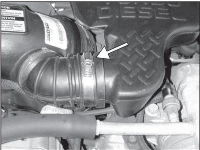
c. Loosen the hose clamp securing the intake resonator to the air intake tube. Remove the intake resonator from the engine bay.
