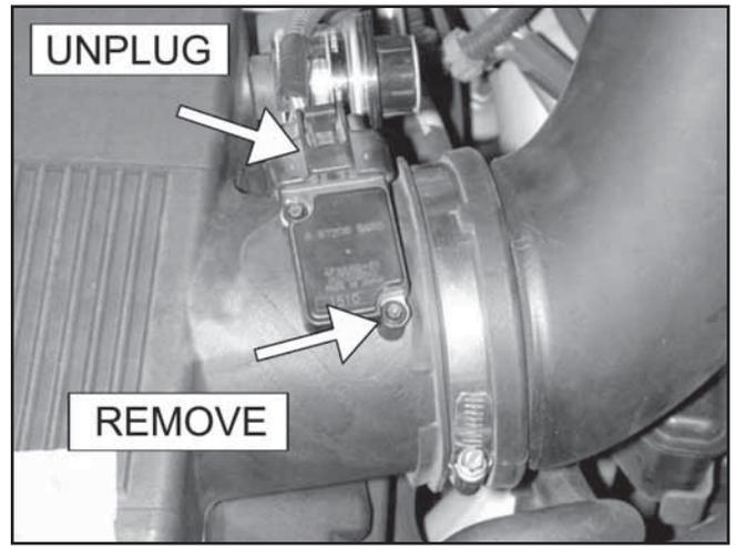
d. Unplug the wire harness from the mass air flow (MAF) sensor. Remove the two screws retaining the MAF sensor with the supplied tamper-resistant Torx tool. Carefully remove the MAF sensor and set aside in a safe area.
