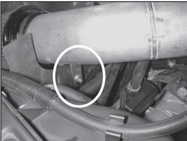
h. The mounting bracket on the AEM® inlet pipe will line up with the rubber mount installed in step 3b. Loosely secure the bracket with the remaining washer and locknut. Refer to the diagram for proper rubber mount installation.
