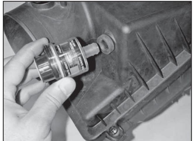
h. Remove the air filter restriction gauge from the factory air box. Make sure the rubber grommet stays in the air box. Reset the gauge by pressing the button on the top.
