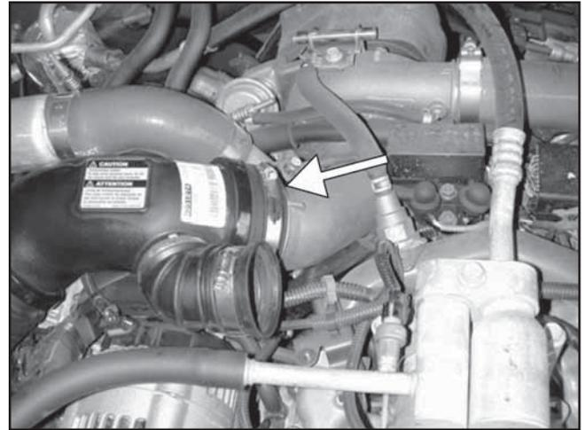
f. Loosen the hose clamp at the turbo inlet side of the air intake tube. Remove the air intake tube from the engine bay.
