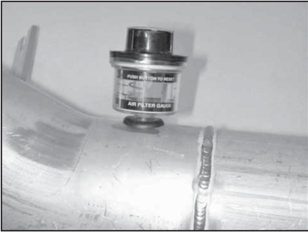
f. Install the supplied rubber grommet in to the AEM® inlet pipe. Insert the air filter restriction gauge into the grommet, being careful not to push the grommet all of the way through the hole.
