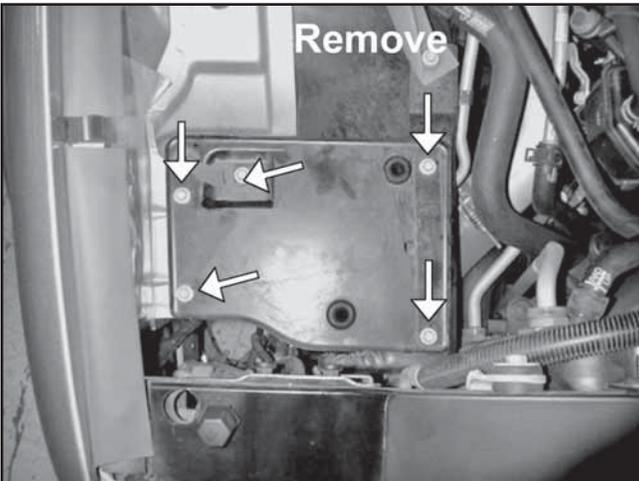
g. Remove the air box by pulling straight up. Remove the air box mounting tray by removing the five bolts. Save the bolts for use during the installation of the AEM® heat shield.
