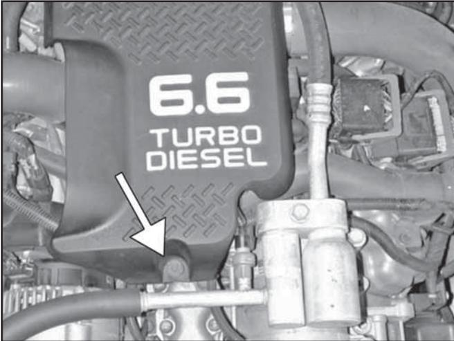
a. On 2001 models, loosen the bolt securing the engine cover, then remove the engine cover. Proceed to step 2d.
