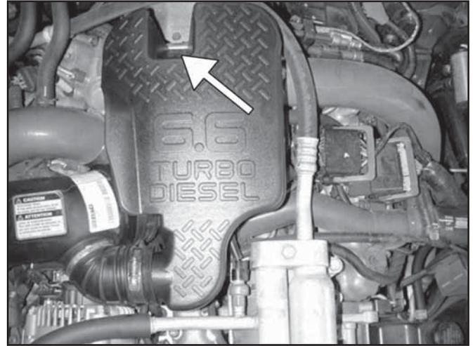
b. 2002 and on models, remove the bolt securing the top of the intake resonator.
