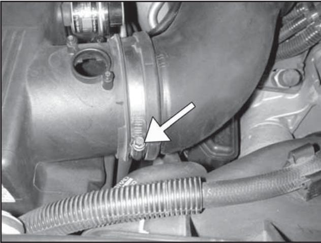
e. Loosen the hose clamp at the air box side of the air intake tube.
