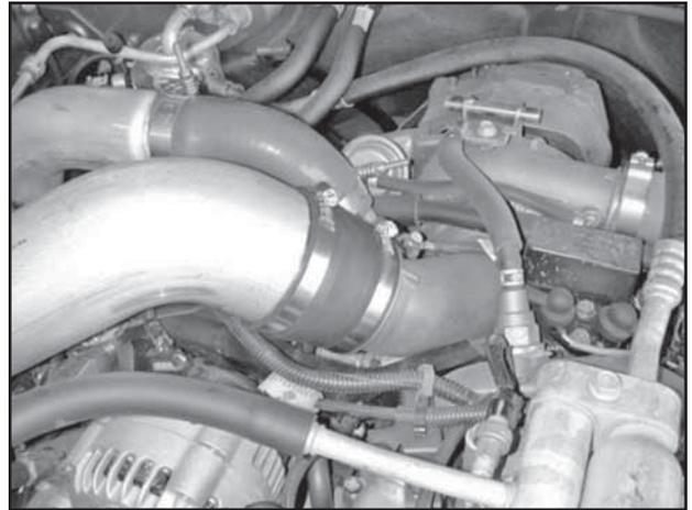
g. Install the open end of the reducer coupler on to the turbo inlet.
