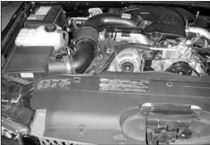
a. Factory air box system.
