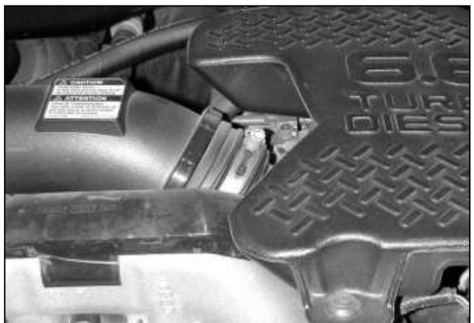
d. Loosen the hose clamp at the turbo inlet side of the air intake tube. Remove the air intake tube from the engine bay.
