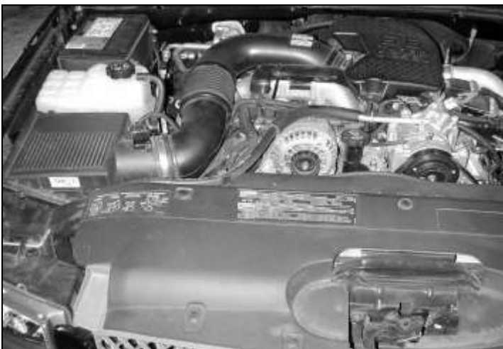
Factory air box system installed
