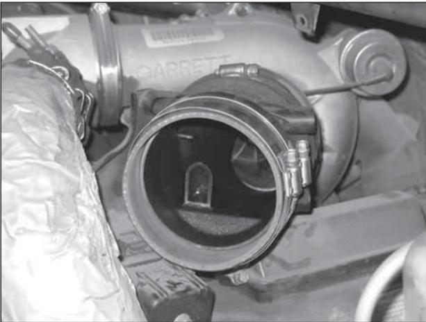
b. Install the 5-402 coupler onto the turbo inlet hose and secure using two #60 hose clamps.
