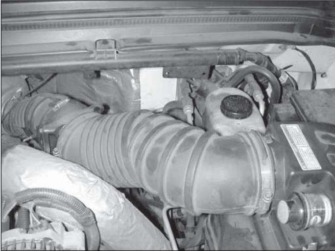
a. Loosen the hose clamps securing the inlet hose to the turbo inlet and the factory air filter housing.
