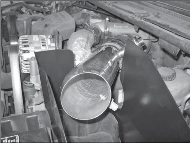
h. Install the intake pipe into the coupler on the throttle body and align the mounting bracket with the rubber mount on the heat shield. Angle the pipe up as shown to gain access to the IAT sensor.
