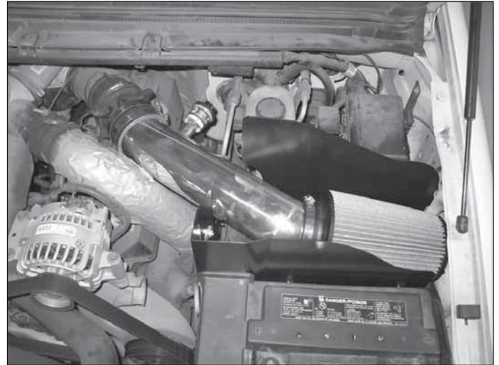
I. Double check the alignment of the pipe, air filter, and heat shield for fitment clearance. Once fitment has been verified, tighten the hose clamps on both the coupler and the air filter. Install the supplied rubber edge gasket onto the top edge of the heat shield now if desired, trim excess.
