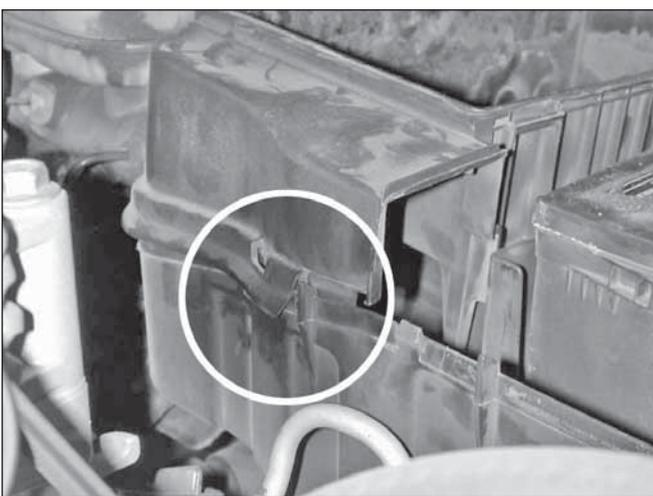
i. Unclip the passenger's side snap of the lower air filter housing. Remove the lower air filter housing.
