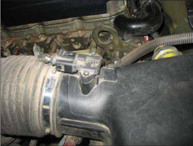
a. Stock air box system. Unplug the wiring harness from the Inlet air temperature (IAT) sensor.
