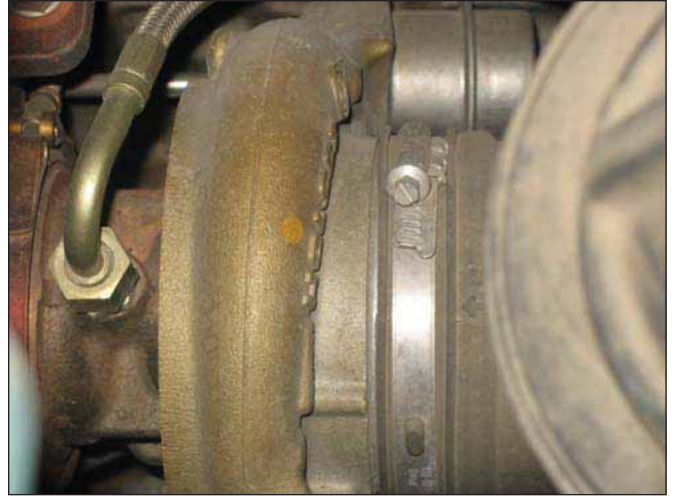
b. Loosen the hose clamps securing the flexible inlet hose between the turbo inlet and the air filter housing. Remove the hose.
