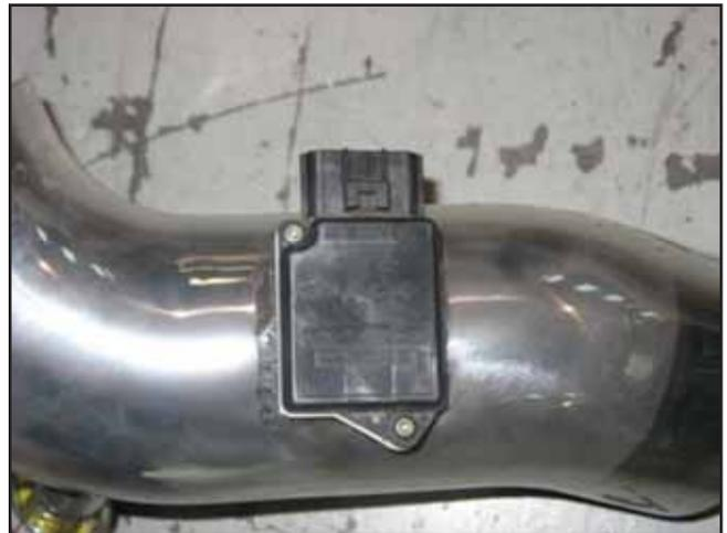
d. On vehicles with a MAF sensor, install the sensor into the intake pipe using the two factory bolts removed in step 2f). If your vehicle is equipped with an IAT, skip to step 3e).
