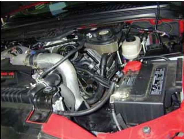
c. Factory air box system removed.
