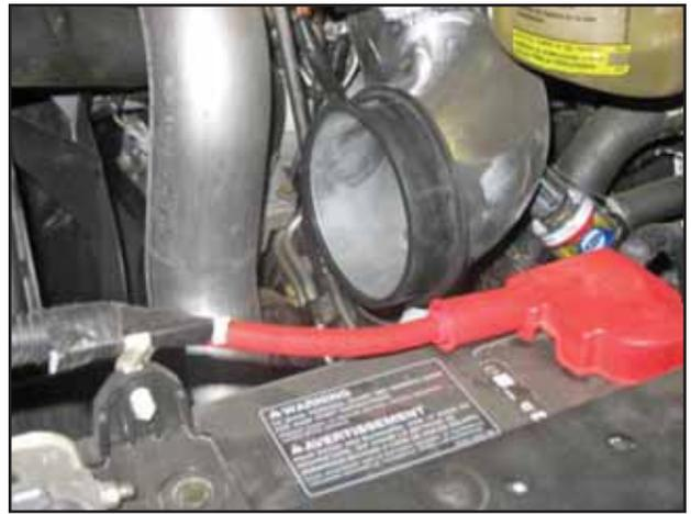
l. Install the supplied air filter adapter by stretching it over the filter end of the pipe.
