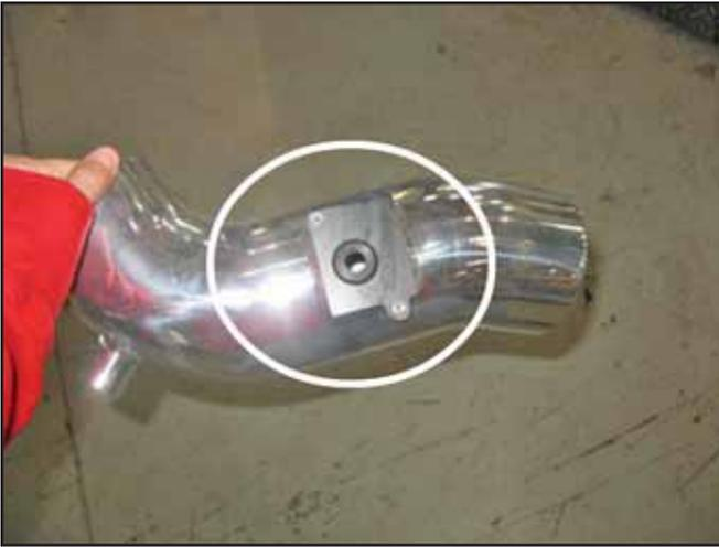
e. On vehicles with a IAT sensor, install provided adapter plate onto the pipe using the two supplied bolts. Install the supplied grommet into the plate.
