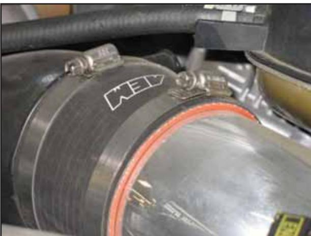
i. Install the pipe into the coupler on the turbo inlet. Align the pipe mounting bracket with the previously installed aluminum stand. Use a #64 hose clamp to secure.
