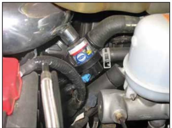
p. Plug the air filter restriction gauge into the wiring harness. Be sure the wiring harness is not touching any hot components under the hood.
