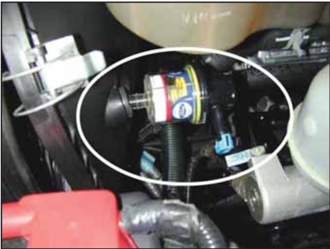
c. Unplug the wiring harness from the air filter restriction gauge. Remove the gauge from the rear of the air filter housing.
