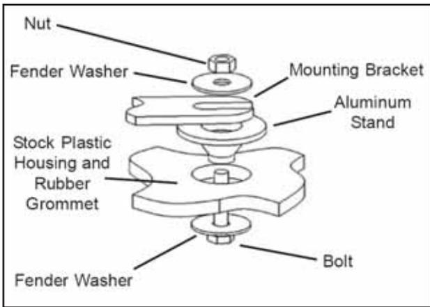
k. Diagram for mounting bracket. Once aligned properly, fully tighten the nut.
