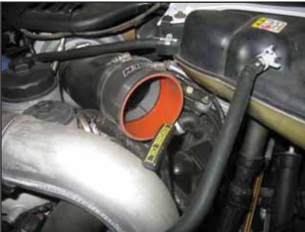
g. Install the silicone coupler onto the turbo inlet and secure using two #64 hose clamps.
