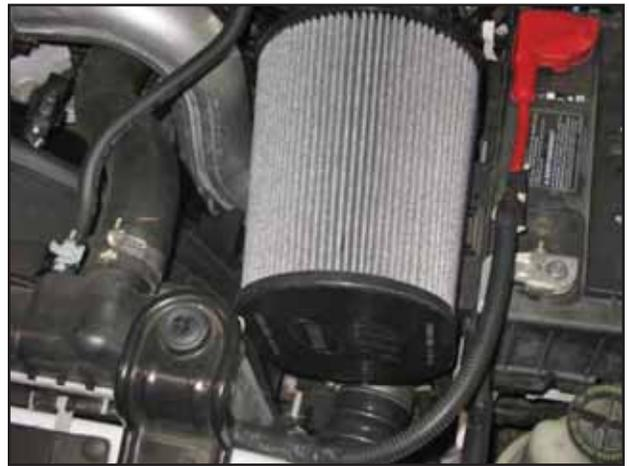
n. Rotate the filter until it is not touching any part of the vehicle and secure it using the remaining #64 clamp.
