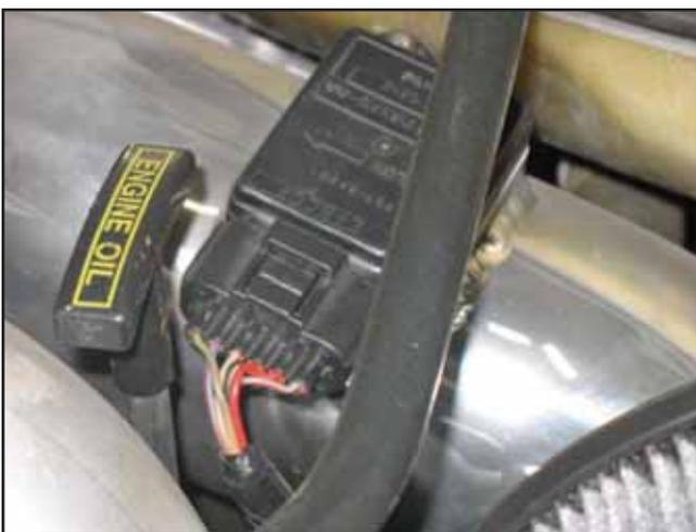
o. Plug the MAF or IAT sensor into the wiring harness. Rotate the oil dipstick for clearance.
