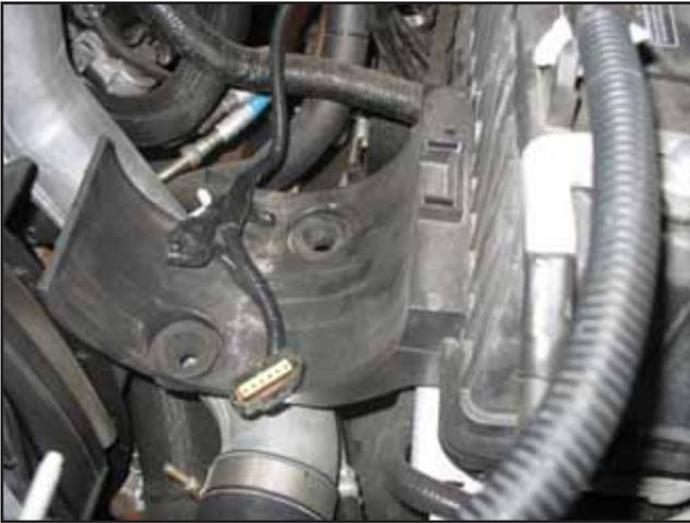
e. Pull up and remove the air filter housing from the engine bay.
