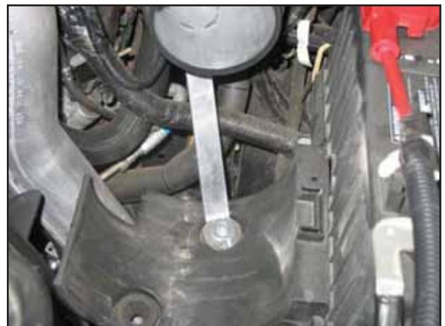
j. Install the supplied M6 washer and bolt through the bottom of the aluminum stand. Secure the bolt using another M6 washer and serrated nut as shown in step 3k.
