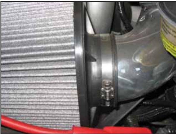
m. Install the Dryflow™ filter onto the filter adapter.
