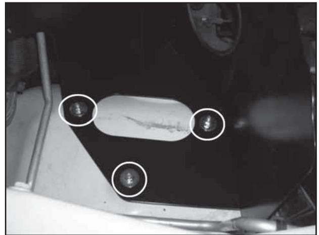
j. Install the three supplied M6 nuts and washers onto the studs from step 3h. Once heat shield is aligned properly, fully tighten the nuts and the bolt from step 3i.
