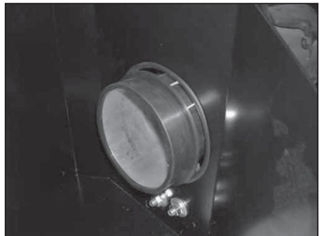
r. Check that the pipe is centered in the heat shield hole. Once confirmed, tighten the nuts on the bracket and the hose clamps on the pipe and turbo.
