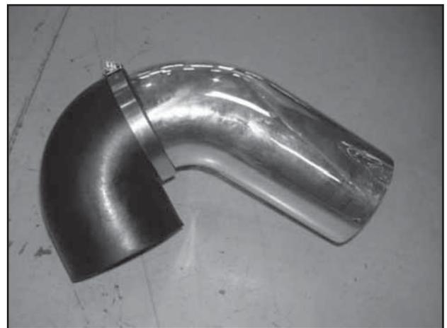
l. Loosely install the 90 degree coupler onto the short end of the pipe as shown. Use a #64 hose clamp but do not tighten it down on the pipe.
