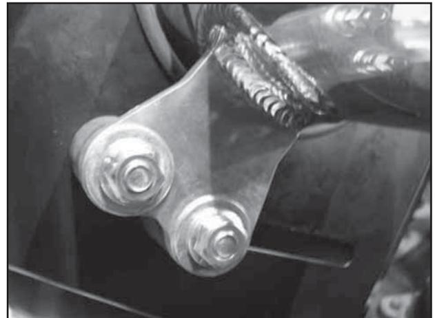
p. Secure the pipe mounting bracket to the heat shield using the supplied M8 washer and bolt.
