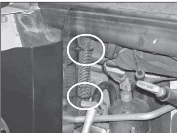
k. Secure the two previously installed zip-ties to the main wiring harness by the vehicle firewall. Trim the excess plastic.
