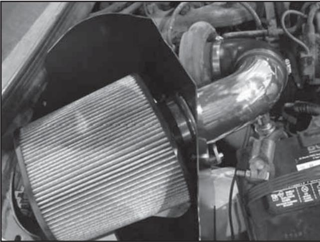
s. Install the Dryflow™ air filter onto the filter adapter. Rotate the air filter until it is not touching any part of the vehicle and secure it using the remaining #64 clamp.
