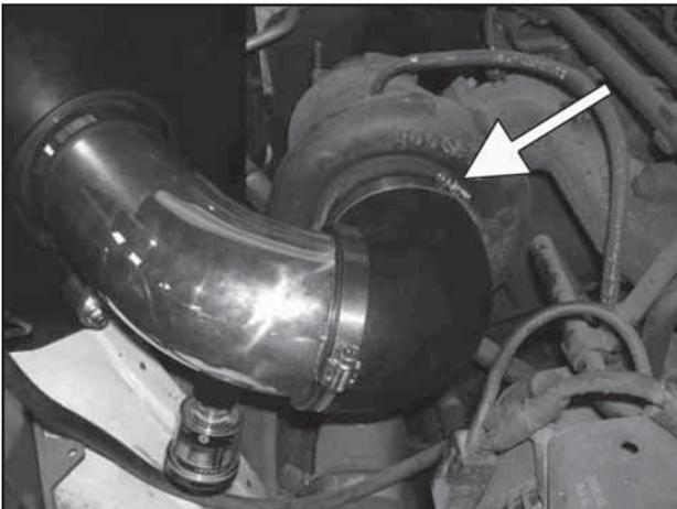
o. Secure the coupler to the turbocharger using a #64 hose clamp but do not fully tighten the clamp yet.
