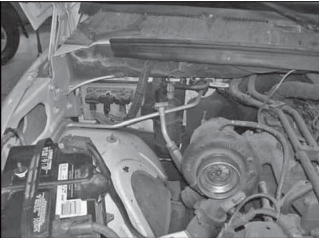
c. Stock intake system removed.
