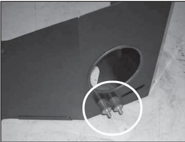
g. Install the two rubber mounts into the two holes on the heat shield using the supplied M8 washers and nuts. Do not tighten the nuts.
