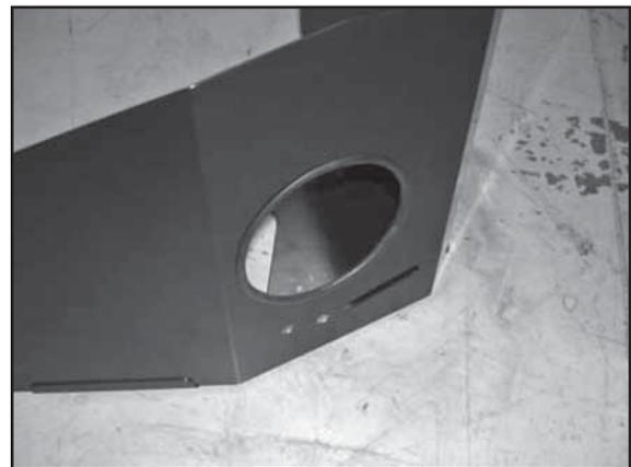
f. Install the supplied rubber edge trim to the hole on the heat shield. Trim to fit.
