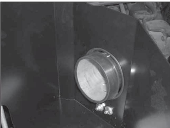
q. Install the supplied air filter adapter by stretching it over the end of the pipe.
