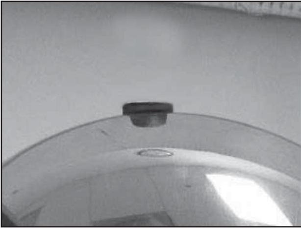
m. Install the grommet (784646) onto the pipe (use soapy water to aid installation). Place the grommet into the pipe at an angle and rotate it until the groove engages the pipe. Reinstall filter minder gauge into adapter.
