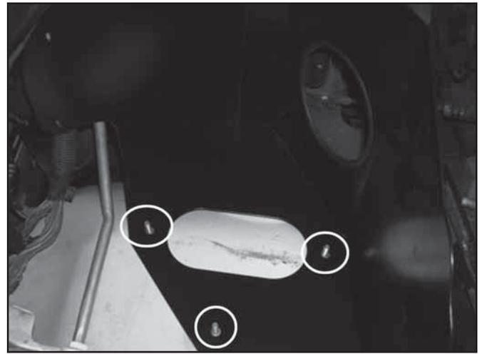
h. Carefully place the heat shield in the engine compartment aligning the three holes on the bottom with the studs in the inner fender.
