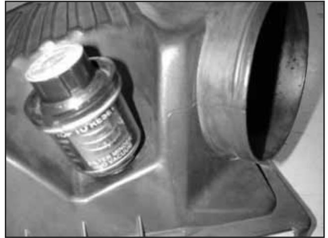
f. Remove the factory air filter restriction gauge from the stock air filter housing lid.
