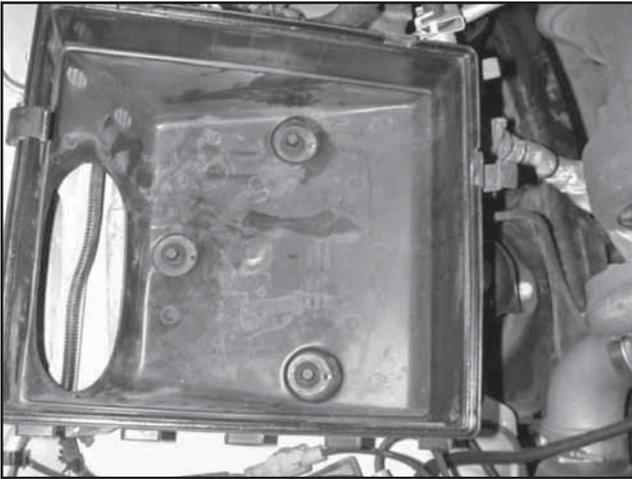
e. Loosen the three plastic nuts securing the lower air filter housing to the vehicle. Remove the housing by gently lifting up.
