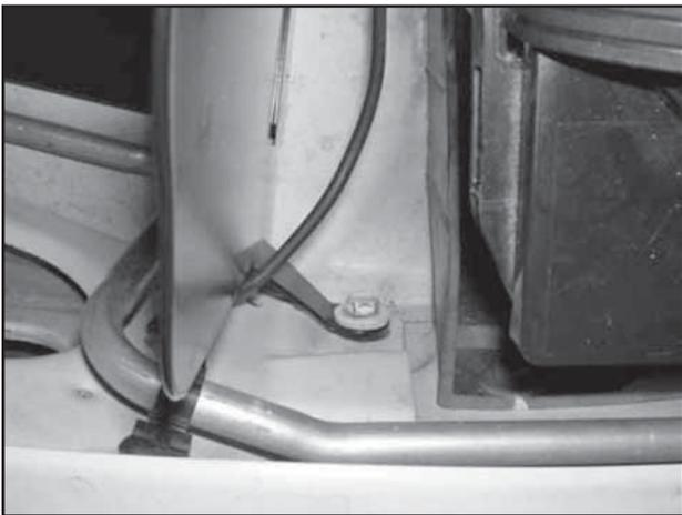
i. Align the small mounting tab with hole where the bolt was removed in step 3c. Reinstall the bolt, securing the heat shield to the inner fender.
