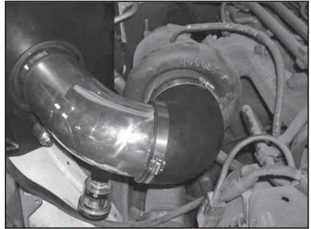
n. Install the intake pipe by sliding the long end of the coupler over the turbo inlet while aligning the mounting bracket on the pipe with the two rubber mounts on the heat shield.
