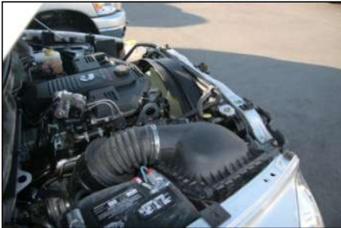
Factory air box system installed
