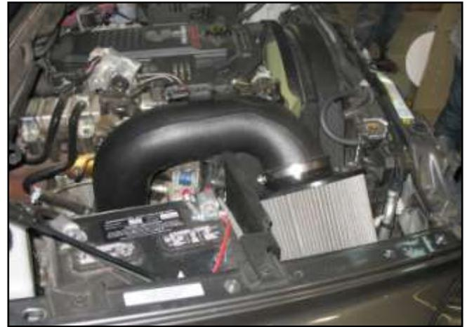
AEM® intake system installed
