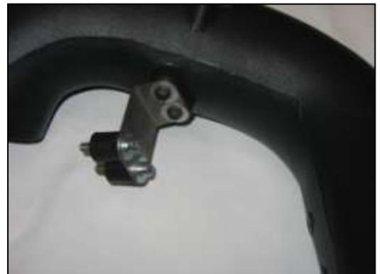
c. Install the included bracket and rubber mounts onto the intake tube assembly as shown, using the included bolts and washers. Do not over tighten.
