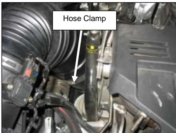
c. Loosen the hose clamp securing the factory inlet hose to the turbocharger. Remove the inlet hose.
