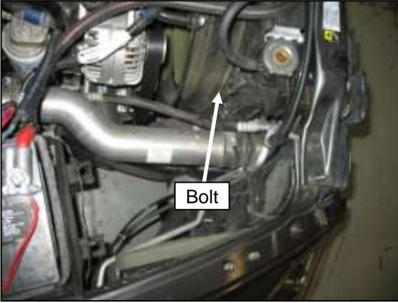
e. Remove the radiator support bolt as indicated. Make a note that the bolt with the pointed end is for the fender.
