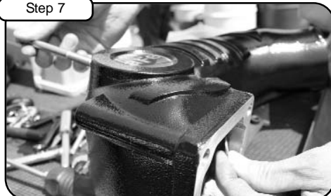
Step 7 Insert the 2 shorter M8 socket cap screws through aFe manifold. Hold washer against inside mounting flange of aFe manifold and feed screw completely through. Insert the two longer M8 screws w/ washers through the outside mounting bosses.
