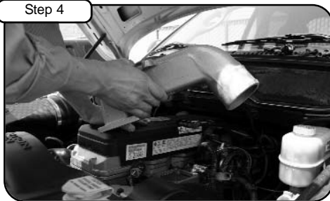
Step 4 Carefully remove stock manifold out of vehicle. ( Place a clean shop rag over air grid heater to prevent anything from entering )
