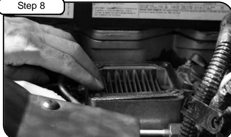
Step 8 Remove both top and bottom stock gaskets away from air grid heater. Replace with new gaskets provided. ( May require a scraper or scotch brite to clean sealing surfaces. )
