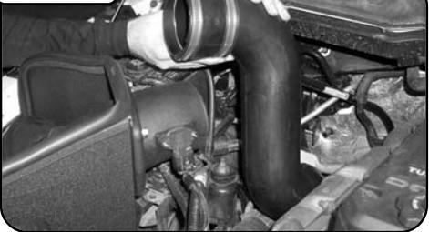
With clamps and couplers provided install high temp coupler at turbo side and 4"x3" urethane coupler at filter side, tighten using 5/16" nut driver. Install pre-oiled filter onto intake tube and tighten. Do not use any oil or grease when attaching filter. Reattach
