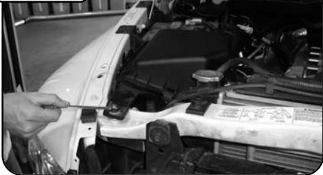
Using 10 mm wrench, remove the bolt that secures the factory airbox to the radiator bulkhead.
