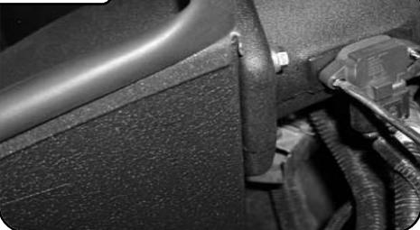
Install intake temperature sensor that was removed from the airbox onto the aFe intake tube using provided hardware and gasket, then tighten. Orientation does not matter on the temperature sensor. Re-connect factory harness to the temperature sensor.
