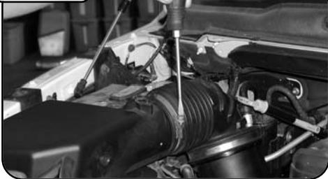
Loosen clamp holding factory tube to factory airbox and clamp at turbo. Remove complete system.
