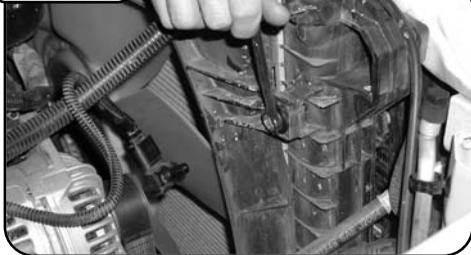
Using a 13mm wrench, loosen and remove the upper passenger-side bolt on the radiator shroud and set aside for installation of heat shield. Verify that the engine is cool, then temporarily remove the overflow hose from the radiator filler neck for clearance.
