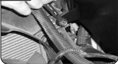
Using the bolt removed from the fan shroud earlier, secure the heat shield to the shroud using the tab extending from the heat shield, do not fully tighten.
