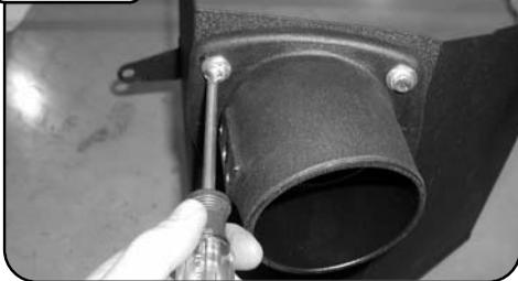
Install aFe intake tube and trim seal on the heat shield, be sure to install in the orientation shown. Install heat shield into engine compartment but do not attach any bolts. The bottom louvered panel must be positioned above the aluminum A/C line.
