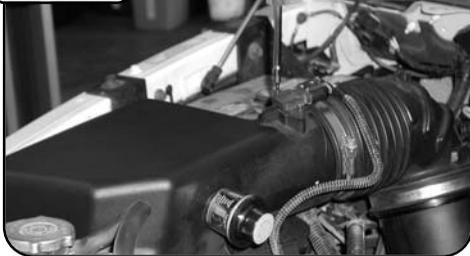
Disconnect the factory wiring harness from the intake temperature sensor located on the top of the airbox. Remove the intake temperature sensor from the airbox and set aside.
