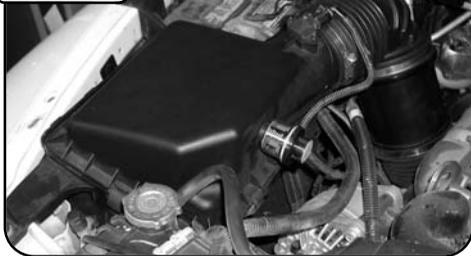
**Complete stock intake.** Make sure that the engine has sufficiently cooled down prior to starting installation of this kit.
