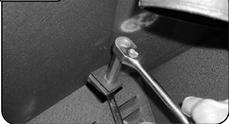
Using provided bolts, locking nuts and washers on both sides of the bolt, fasten lower tab on heat shield and slotted hole to the existing rubber mounts. Be careful not to over-tighten, it is only necessary that the rubber mounts be slightly compressed. Fully tighten shroud.
