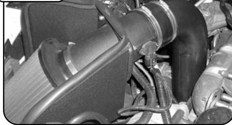
**Complete intake kit installed.** Be sure to re-check connections and re-tighten after a few hours of operation. Thank you for choosing aFe!
