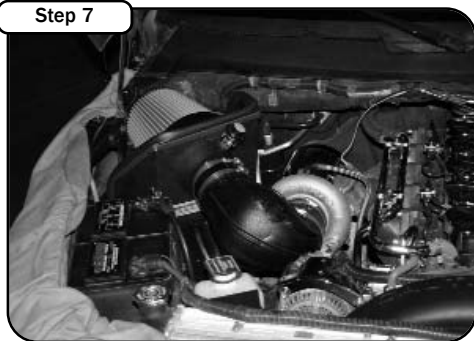
Your installation is now complete. Make sure all clamps are tight and that all electrical components are secure. Check and retighten connections after a few hours of operation.
