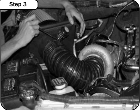
Loosen the two hose clamps on the intake duct. Remove intake duct out of the engine bay.
