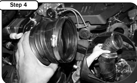
With 5/16" nut driver, loosen the clamp at air box and at bottom of intake tube. ( Make sure NOT at turbo! ) Remove upper half of OE intake tube and leave bottom OE coupler.
