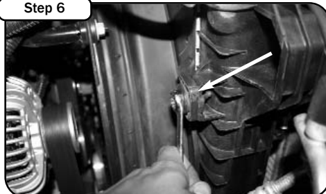
Loosen and remove the 13mm radiator bolt. Set aside for later use.
