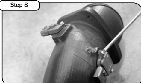
Insert MAF sensor and temp sensor into new tube with gaskets and #8-32 screws provided. Tighten using flathead screwdriver.
