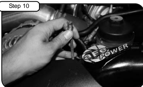
Step 10 Install and secure manifold using 2 M6 x 1.00 x 100 screws and washers provided and tighten loosely.
