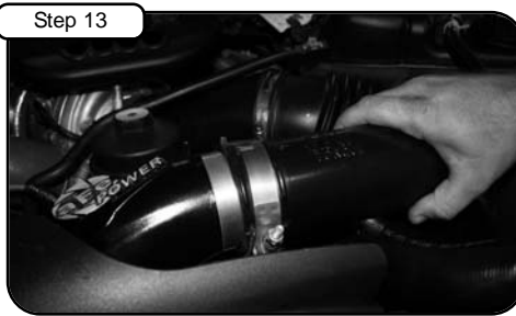
Step 13 Re-attach intercooler tube to manifold.
