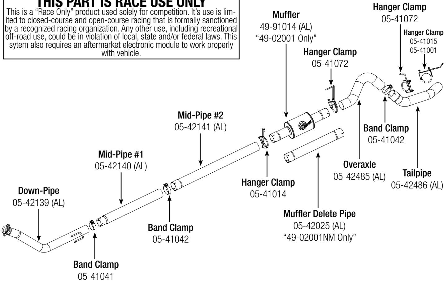
**Step 1: (Read Instructions prior to installation)** Remove the stock exhaust from the rear of the truck working your way forward. It may be necessary to cut the pipes if the slip joints are stuck. Take caution not to damage the factory isolation mounts as they will be reused. Disconnect sensors at the connections. Take caution as not to damage any sensors. **It is recommended to not fully tighten the clamps until the entire system has been installed.**
