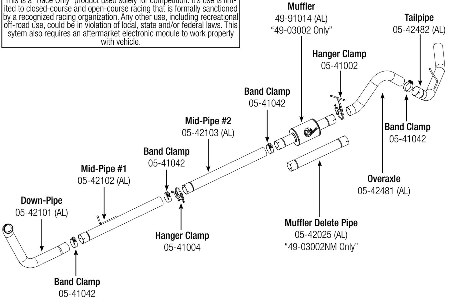
**Step 1: (Read Instructions prior to installation)** Remove the stock exhaust from the rear of the truck working your way forward. Take caution not to damage the factory isolation mounts as they will be reused. If you want to remove the OE downpipe in one piece or without cutting, you must remove the transmission cross member and disconnect the dip-stick tube and sway bar end links. **It is recommended to not fully tighten the clamps until the entire system has been installed.**
