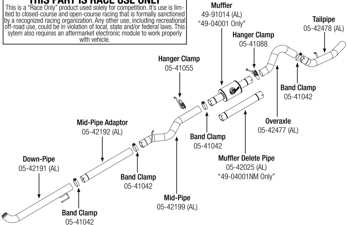
**Step 1: (Read Instructions prior to installation)** Remove the stock exhaust from the rear of the truck working your way forward. It may be necessary to cut the pipes if the slip joints are stuck. Take caution not to damage the factory isolation mounts as they will be reused. **It is recommended to not fully tighten the clamps until the entire system has been installed.**
