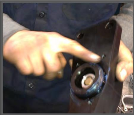
10. WITH ASSEMBLY GREASE OR LIGHT OIL, LUBRICATE THE SEALING RING OF THE FLEECE PERFORMANCE THERMOSTAT HOUSING, AND PRESS IT INTO PLACE ON THE BACK OF THE ENGINE BLOCK. THE -10 COOLANT LINE SHOULD BE ORIENTED TOWARDS THE PASSENGER SIDE, AND OVER THE EXHAUST MANIFOLD.
