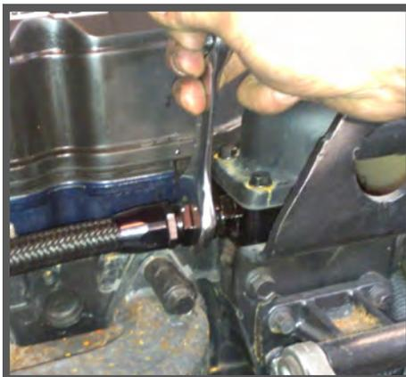
12. WITH THE COOLANT LINE ROUTED ABOVE THE EXHAUST MANIFOLD, CAREFULLY THREAD THE AVAILABLE END ONTO THE AN STYLE FITTING OF THE THERMOSTAT RISER BLOCK.
