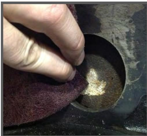
8. WITH THE FREEZE PLUG REMOVED, USING A SCOTCH-BRITE™ PAD AND A DEGREASING SOLUTION, THOROUGHLY CLEAN THE BLOCK SURFACE AREA FROM THE HEAD DOWN TO THE REAR COVER, AS WELL AS THE BORE WHERE THE FREEZE PLUG WAS PREVIOUSLY INSTALLED. BE SURE TO REMOVE ANY DIRT OR FOREIGN DEBRIS.
