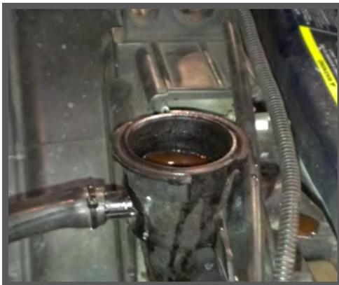
14. ENSURE THAT THE DRAIN PLUG HAS BEEN SECURED IN THE RADIATOR, AND PROCEED TO RE-FILL. IT WOULD BE A GOOD OPPORTUNITY TO REPLACE THE COOLANT AT THIS TIME. HOWEVER IF A CLEAN DRAIN PAN WAS USED, THE COOLANT CAN BE REUSED. BE SURE TO REMOVE ANY POSSIBLE FOREIGN DEBRIS.
