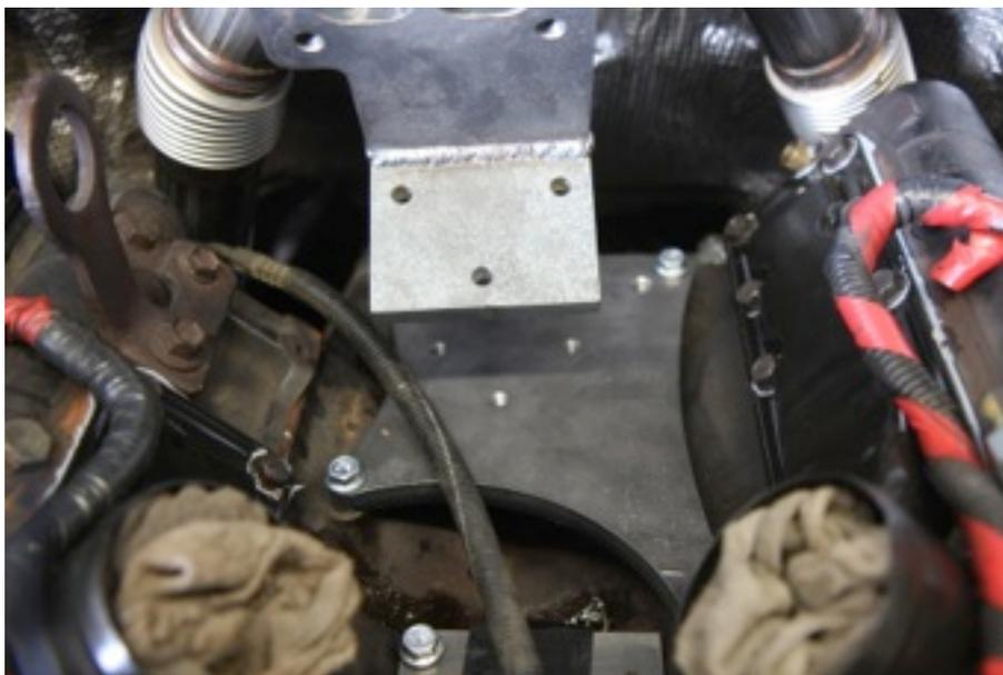
6. Instal the 8x60mm bolts from the flanges on the up-pipes to the manifolds. When all are install then tighten the bolts down.
