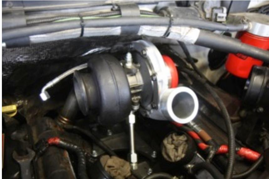
9. Install the upper portion of the downpipe to the turbine discharge, slide up the lower portion of the downpipe and attach with clamp. Align the downpipe into position and tighten down the clamps.
