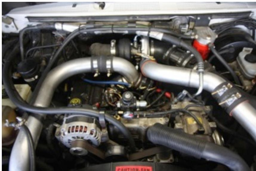
12. attach air intake system to protect the turbo from ingesting foreign debris.
