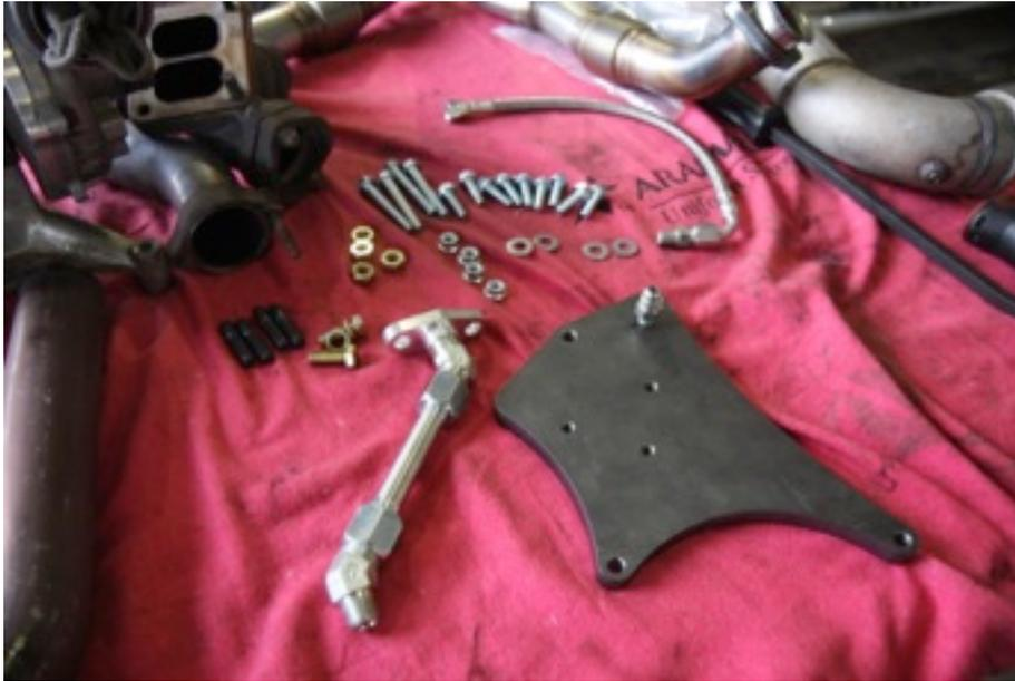
4. Then install the 1/8NPTx6JIC fitting supplied, put a couple wraps of teflon tape around threads to help lubricate the threads for install (pictured above).
