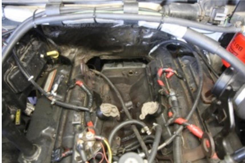
2. If installing turbo on Superduty truck remove the soft plug from the valley and install the oil drain fitting using two supplied 8x25mm bolts. If installing in a superduty then the soft plug in the valley needs to be removed. This can be done by drilling a small hole and then installing a screw into the hole and grabbing with pliers to ensure it doesn't fall into the motor. It may be necessary to tap gently to break it loose.
