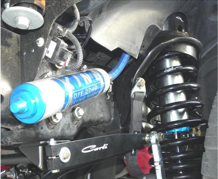
25. Install Sway-Bar Drop-Forward Brackets to the frame with factory hardware. Gussets will face the inside, smooth side out and the brackets will drop the sway bar down and FORWARD.
