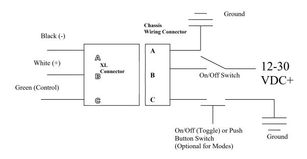
When using the optional On/Off (Toggle) or Push Button Switch, depressing the switch will dim the light to 50% power. Depressing the switch again will toggle back to full power.
