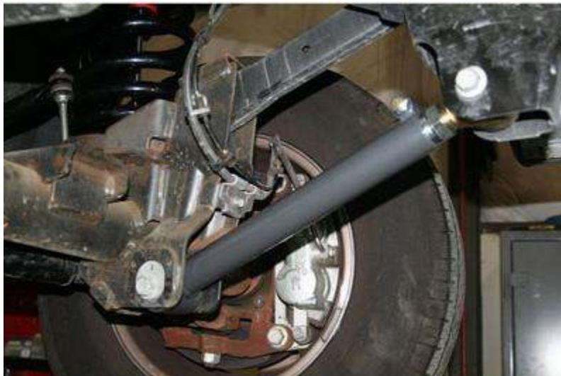
5. We recommend presetting the length of the lower control arm. For 3" lift, we recommend a length of 19" measured from center to center of the bushings. This length is a good starting point when using the stock length upper control arms. The final length should be adjusted to get the correct amount of caster. Approximately 3-5 degrees is the factory spec. We suggest shooting on the higher end of the range for improved straight line tracking and vehicle return to center.
