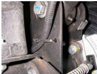
48. Remove the bolt that holds the brake line to the frame. This will allow the axle to droop far enough to get your six-inch springs in.
