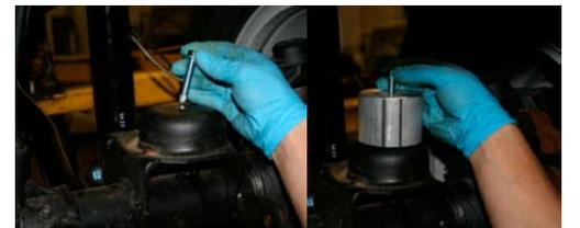
39. Install the new front springs. Using a coil spring compressor can make this easier.
