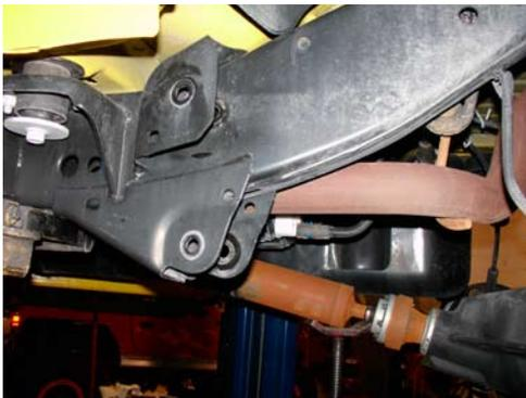
12. Remove both front upper and lower brackets and grind the remaining weld smooth with the frame in preparation for installing the new combination front bracket.
