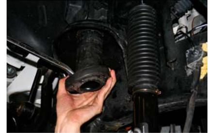
34. Install the new front spring spacer.
