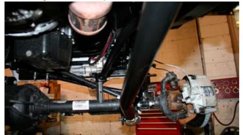
18. The front upper arms require lifting the engine about one inch to get the provided 9/16"x3" bolt in on the frame side. The engine mounts are slotted, making it so that you can loosen the two main bolts and lift the engine about an inch. Use the bottom of the two holes for most applications. Position grease zerks for access and where they will be most protected from rocks or other damage. Set front upper arm length to 28 1/16".
