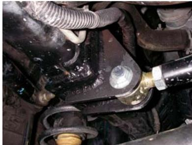
Make sure the bracket fits the frame and is in the proper location. Tack two or three places to keep the bracket from pulling during final welding. Remove the brace and then final weld the rest of the bracket. *A professional certified welder is always a good way to go if you have any doubts about your welding ability.*
