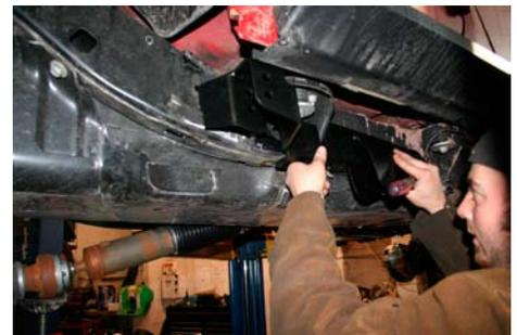
On the driver side hold the bracket into place. *There is no hole to match up the to on the frame so the exact location should be determined by measuring the other side and matching the driver side to it.* Mark the bracket and the frame for welding preparation. Remove the bracket and clean off the paint from the bracket and the frame
