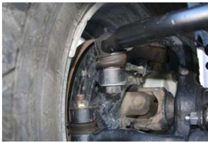
45. Reinstall the breather hose if it was disconnected during disassembly.
