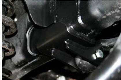
28. Tighten the bolts that go in the steering box and the 1/2" button head bolt.
