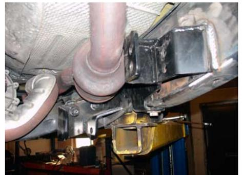
16. After the welds have cooled, clean the frame and brackets. Paint over welds and any other raw metal areas left from grinding and sanding.
