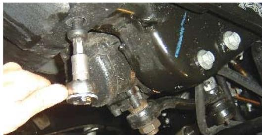
31. Hold the steering box skid plate in place, make sure that the holes line up.
