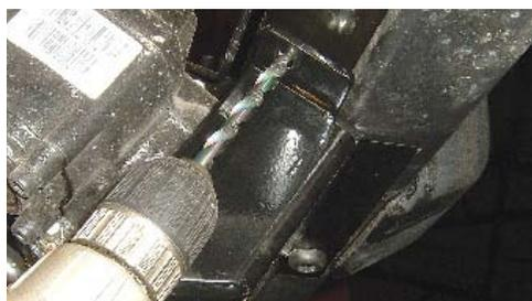
34. Use a 5/16" drill bit to drill the frame at the location you just marked.
