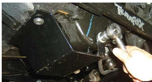
**Note:** Use flat washers to correct the spacing of skid plate when using stock bumper if necessary.
