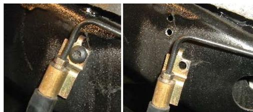
38. Line up bracket with holes in the frame so the bracket extends down.
