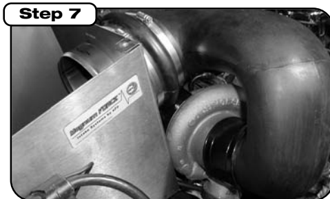
Slip boots over intake tube and install on turbo and filter housing. It may be easier to install clamps after tube is in position. If filter restriction gauge is desired, drill an 11/16 hole with a woodworking spade bit and transfer grommet and sensor to new intake tube. Sensor should be placed near larger end of tube for accurate results.
