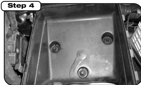
Remove lower half of filter box, unscrew 3 inserts and transfer inserts to new filter housing.
